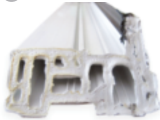
After Welding Corner Cut Open
